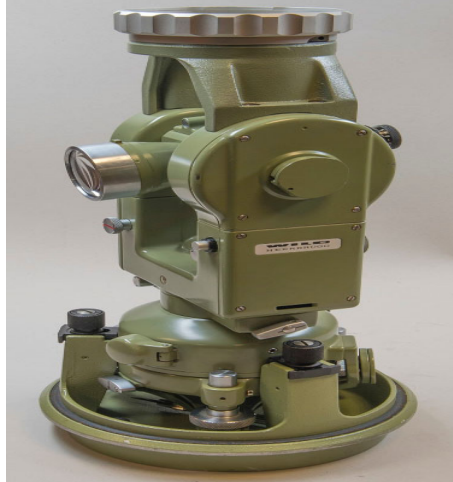
Fig 2.33 - Wild T2 theodolite developed by Heinrich Wild in 1919
